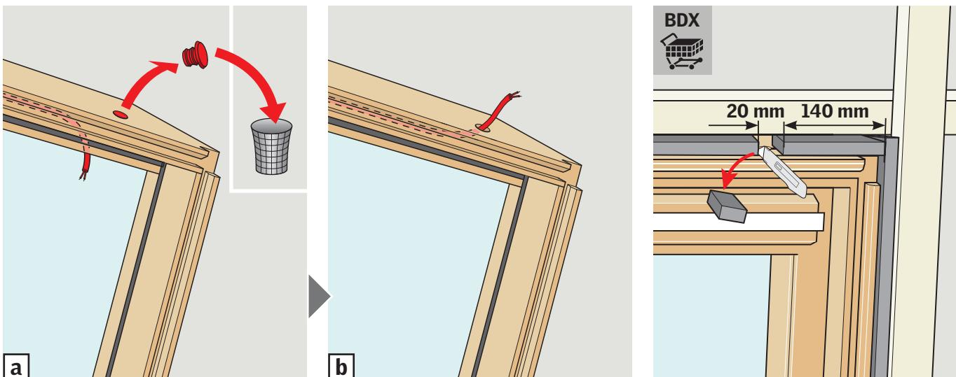
**ENGLISH:** Remove cover cap (**a**). Run cable through the pre-drilled hole (**b**) and extend by using fire rated cable to control system KFX. The window operator is a 16-30 V DC product and must not be connected directly to the mains as this will damage the motor.
