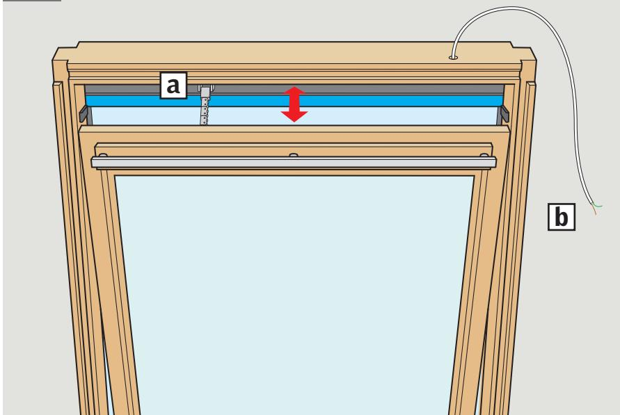
**ENGLISH:** Extend the chain to its full length (this requires power for the window operator). Connect the chain to the chain bracket using the retaining clip which must be inserted **from the right to the left** as shown (a). Close the window (requires power for the window operator). The window is now ready for use.
