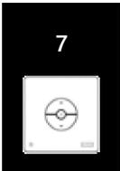
**7** Push the 'pair' button on the bottom of the wall switch for 1 second.
